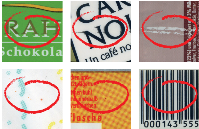
All defects, such as color spots, printing deviations, inclusions in paper or contaminations, are reliably detected and classified by the systems.
